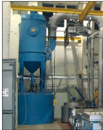
Wet scrubber VDN-T with water holding tank
