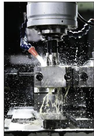
Water-soluble aerosols are released from coolants during cutting processes.
