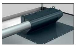
ProChip is installed on top of the machine housing.
