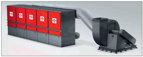
Central separator consisting of five AERO® modules of size 3 and one fan (nominal air flow of 64 000 m³/h)
