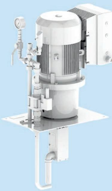
Screw pumps are displacement pumps. Because of their design, pressure must be limited in order to maintain a reasonable motor current. In addition to burst protection, pressure relief valves ensure that the preset pressure is maintained. Using damped valves in screw pumps prevents pressure surges. In case of overpressure, unnecessary material is discharged through the valve.
