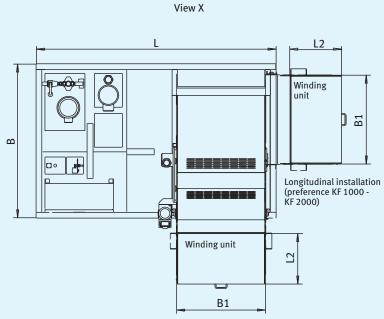
Transverse installation (KF 1000 - KF 2000) Only separate transport possible
